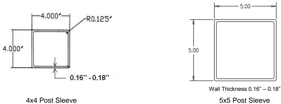
Figure 3 – TAM-RAIL® Post Sleeve Cross Sections
